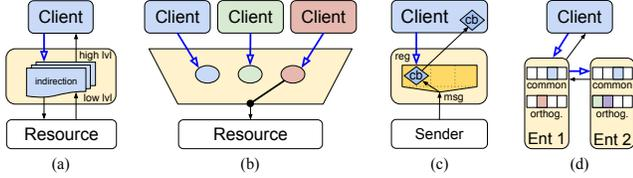
**Figure 2: Common design patterns that cause state spill ( $\rightarrow$ ).** (a) **Indirection Layers** cause state spill when converting between two representations of data/commands; (b) **Multiplexers** harbor state spill when serving multiple clients; (c) **Dispatchers** harbor state spill by holding registered callbacks (cb) for message/event delivery. (d) **Inter-entity collaboration** causes state spill when non-orthogonal states must be synchronized.
